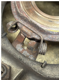
The last two photos show the fitting of the springs on the outer face of the clutch cover (off—left and on-right)
